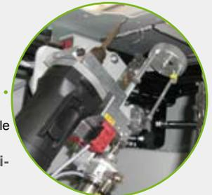
Drill- /milling unit from the bottom with angle adjustment 0-65°.
