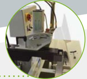
Drilling- / milling unit top with angle adjustment +/-20°.
