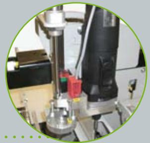
Drilling- / milling unit top with 6-fold revolver stop.
